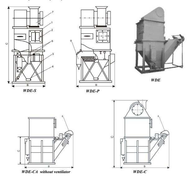
WDE-S - are equipped with the device 4 for a mud discharge;
