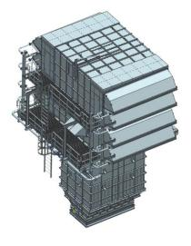
The project Filter House with a 2-sided inlet, for GT-75-80 MW.
