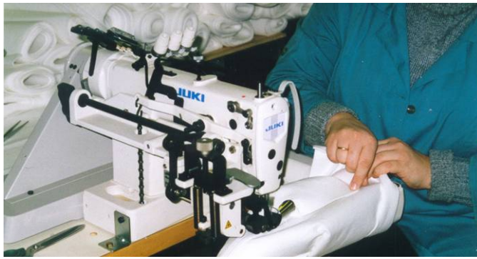
Fig. 2 Specialized sewing machine, providing lock seam
