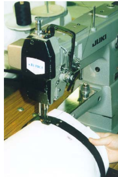
Fig .3 Specialized sewing machine for sewing in rings, pads, etc.
